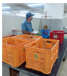
Figure 28: Measuring the specific gravity by potato gauge.
